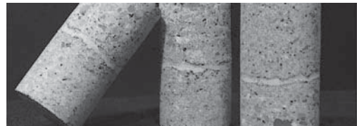
Figure 1. Sample cores of a fully bonded spray applied membrane sandwiched between two sprayed concrete layers.
