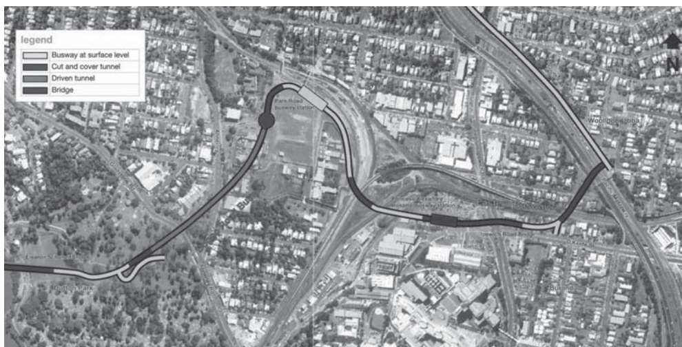
Figure 2. Plan of Boggo Road Busway and Eastern Busway alignment, driven tunnel on left below bus turning bay.
