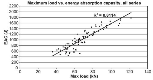
Figure 8. Maximum load versus energy absorption capacity, all series.
