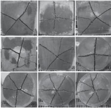
Figure 4. Different crack patterns; 4, 5 6 and 7 cracks appear, examples from different series.
