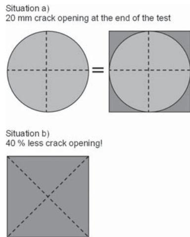
Figure 6. Possible crack patterns, four perpendicular cracks.
