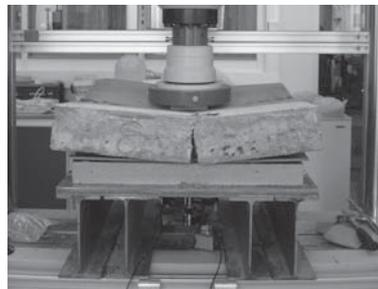
Figure 2. Set-up for square panels. Support of steel, strips of plywood as bedding material.
