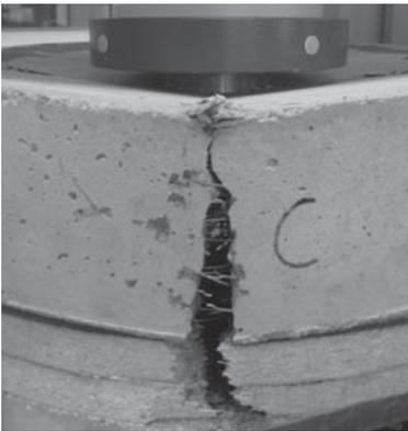
Figure 5. Failure in chipboard support.
