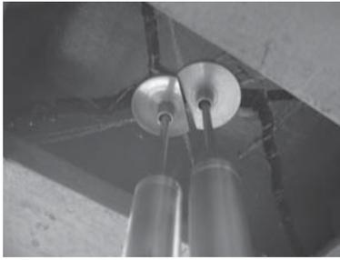
Figure 3. Placing of the two displacement transducers with metal caps.
