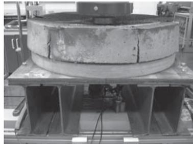
Figure 1. Set-up for round panels. The support fixture was made of plywood of birch/chipboard, no bedding material
