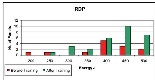
Figure 3. ASTM C1550 round panel energy absorption at 40 mm.
