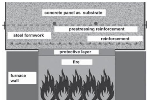
Figure 9. Cross section of a test specimen with protective layer on the oven.
