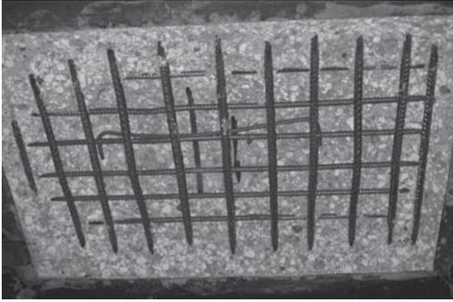
Figure 2. Reinforced concrete test panel after fire ingress showing heavy material loss due to spalling (Kusterle 2004).
