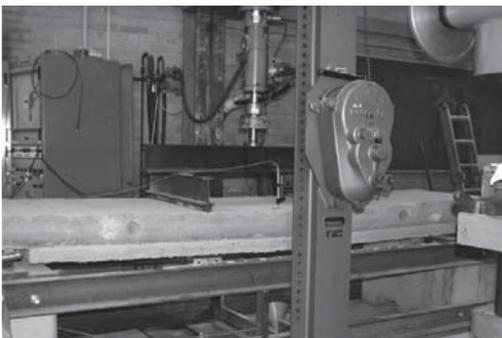
Figure 8. Bending test to demonstrate crack opening in protective layers (picture: Saxer).
