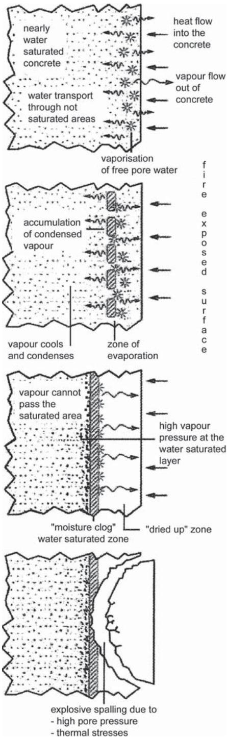
Figure 3. Schematic illustration of water vapour flow within a concrete structure heated from one side (Schneider & Horvath, 2002).
