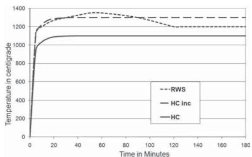
Figure 1. Temperature-time curves which have to be applied for testing and design according to OEVB (2005), OEVB (2006) in Austria (HC and HC increased for hydrocarbon fires with different duration, if detailed fire design is not performed, RWS (Rijkswaterstaat, a Dutch requirement) for proving fire resistance class BBG (fire resistant concrete tested in large scale test, "Beton erhöhter Brandbeständigkeit geprüft im Großversuch") and for protective layers).
