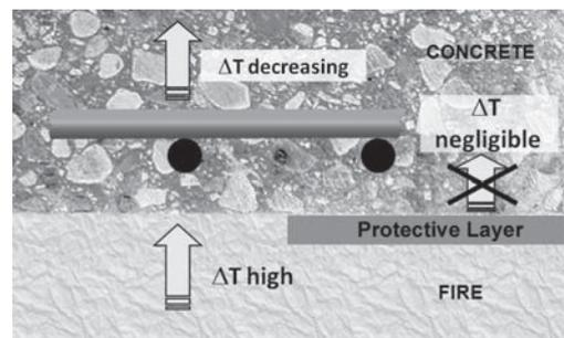
Figure 4. Reduction of the temperature gradient induced by fire to subcritical values by means of a protective layer.
