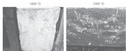
Figure 6. Example of a protective layer after a fire ingress of 1200 and 1350 degree Celsius.
