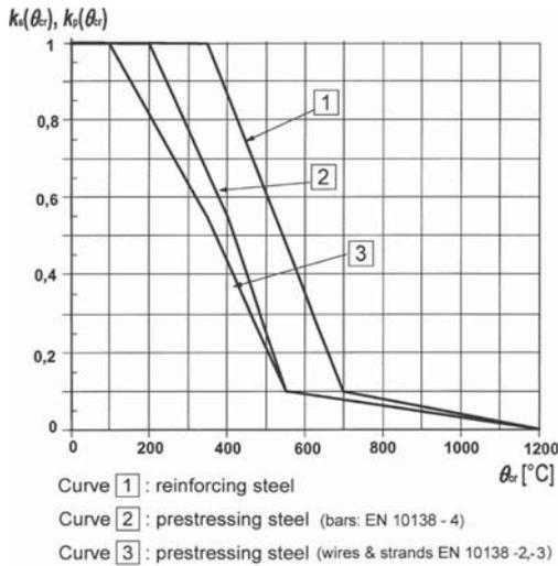
Figure 5. Reference curves for critical temperature of reinforcing steel  $\theta_{cr}$  corresponding to the reduction factor  $k_s(\theta_{cr}) = \sigma_{s,fr} / f_{yk}$  (20° Celsius) or  $k_p(\theta_{cr}) = \sigma_{s,fr} / f_{pk}$  (20° Celsius) according to (EN 1992-1-2, Fig. 5.1, 2007),  $\sigma_{s,fr}$  steel stress in fire situation.
