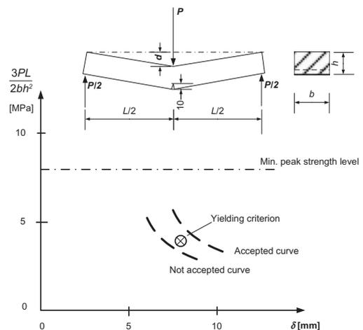
Figure 2. Early Swedish method for defining requirements for steel fibre reinforced shotcrete (the JH method).
