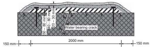
Figure 3. The Swedish drain consists of a perforated plastic tube at the water bearing crack, which is covered by an insulating sheet with closed pores. The sheet is fixed to the rock by short bolts and reinforcement bars. The sheet is covered with steel fibre reinforced shotcrete which bonds to the rock surface at the edges. Finally the steel fibre reinforced shotcrete is covered by unreinforced shotcrete.
