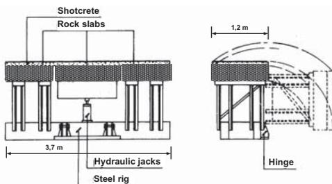
Figure 1. Large scale test rig for experimental investigation of the mode of action of shotcrete bonded to hard rock.
