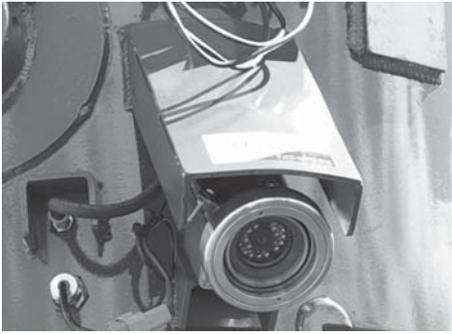
Figure 5. Infra red camera mounted on robot.
