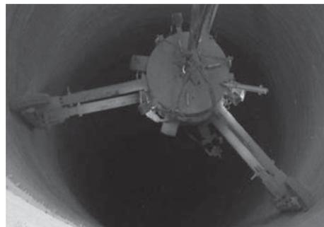
Figure 6. Shaft liner robot suspended in shaft during commissioning.
