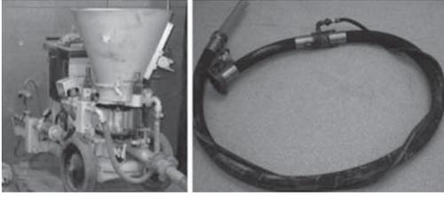
Figure 3. Dry-mix gun and nozzle.
