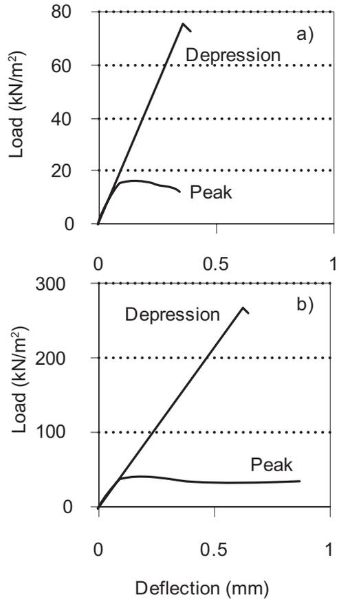
Figure 14. Load-deflection for shotcrete slab with multiple bolts and a thickness of a) 40 mm and b) 80 mm (Nilsson 2004).
