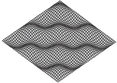
Figure 3. Finite element model of a plane shotcrete slab with harmonic irregularities.
