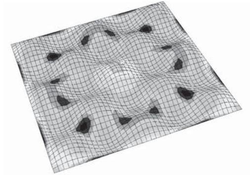
Figure 12. Principal stress distribution on the upper surface of a 80 mm thick shotcrete slab. High tensile stresses around the bolt placed in a depression within the slab (Nilsson 2004).
