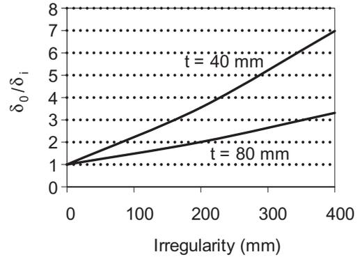
Figure 10. Relative stiffness as a function of irregularity and shotcrete thickness (Nilsson 2004).
