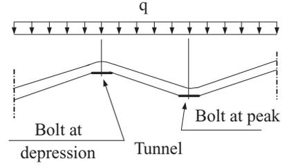
Figure 9. Placement of rock bolts at peaks or in depressions (Nilsson 2004).
