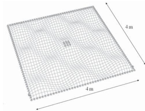
Figure 8. Finite element model of shotcrete and one rock bolt (Nilsson 2004).
