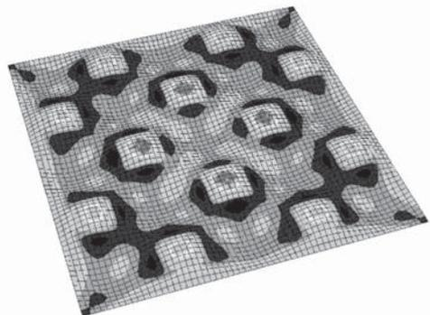
Figure 15. Principal stress distribution on the upper surface of a shotcrete slab suspended using twelve rock bolts. High tensile stresses around the bolts placed in depressions of the slab (Nilsson 2004).
