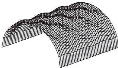
Figure 4. Finite element model of a shotcrete shell with harmonic irregularities.
