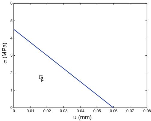
Figure 7. Tensile stress-displacement relationship for the analyzed fibre reinforced shotcrete.
