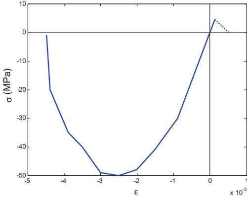
Figure 6. Uniaxial stress-strain relationship for the analyzed fibre reinforced shotcrete.
