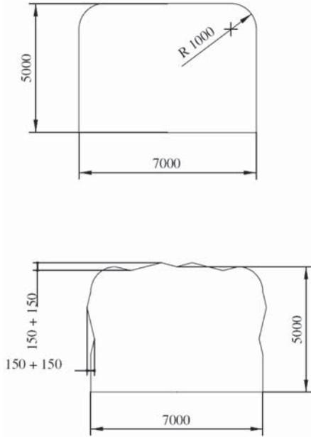
Figure 2. Tunnel with smooth rock surface and with a roughness of 150 mm (Malmgren 2005).
