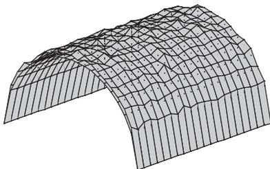
Figure 5. Finite element model of a shotcrete shell with a highly irregular outside and a smooth inside.
