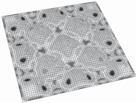
Figure 16. Principal stress distribution on the upper surface of a shotcrete slab suspended using twelve rock bolts. Low tensile stresses around the bolts placed at peaks on the slab (Nilsson 2004).
