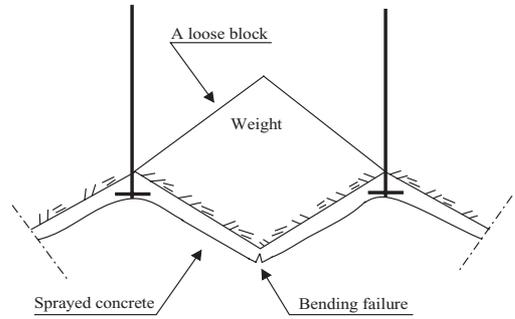
Figure 1. Failure in a bolt-supported shotcrete lining on rock (Chang 1994).
