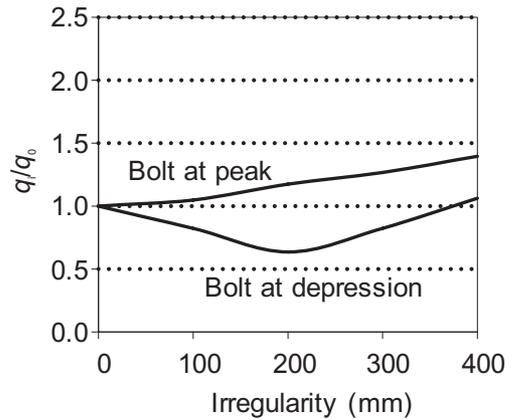
Figure 11. Failure load for a 80 mm thick shotcrete slab as function of irregularity and placement of rock bolt (Nilsson 2004).
