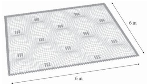
Figure 13. Finite element model of shotcrete and twelve rock bolts (Nilsson 2004).
