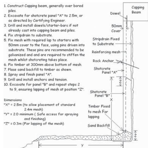
Figure 23. Suggested target shotcrete profile sequence for top-down construction. [Disclaimer: The intention of this profile is to demonstrate the best case scenario in terms of safety, productivity, cost and final finish when constructing walls in a top down nature. Final design and staging should always be checked and directed by a qualified engineer prior to commencement.]
